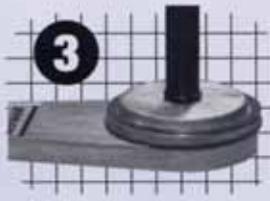
O-ring secures bottom core holder in place when changing film rolls.
